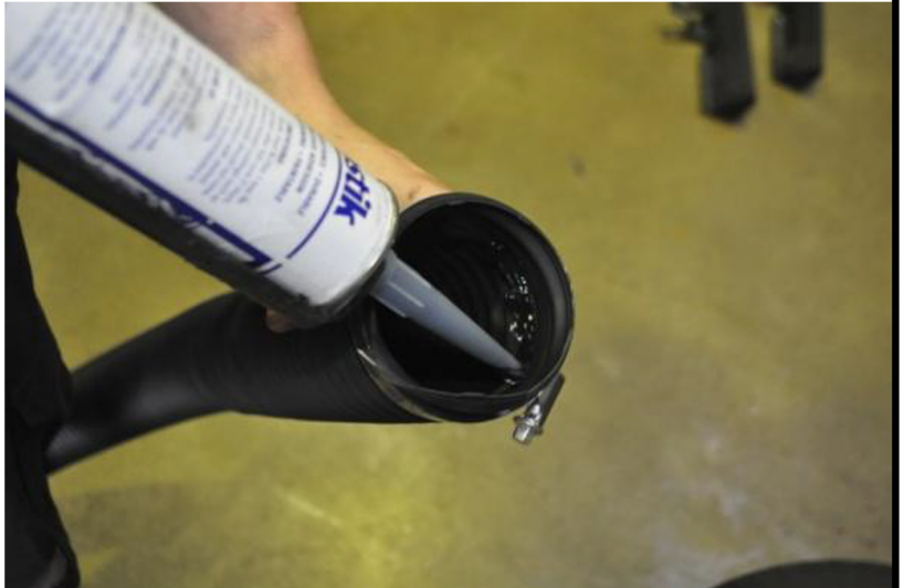
ABOVE: The flexy hose zip tied in the wheel arch BELOW: Don't forget to silicon the air box end of the hose
