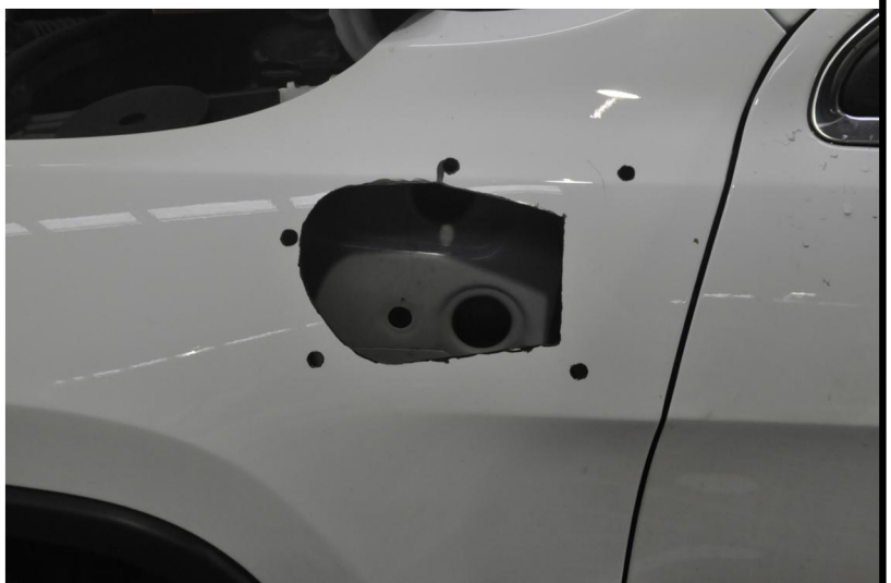
ABOVE: Before: Holes marked for drilling and the cut-out marked out BELOW: After: Holes drilled and the cut-out completed
