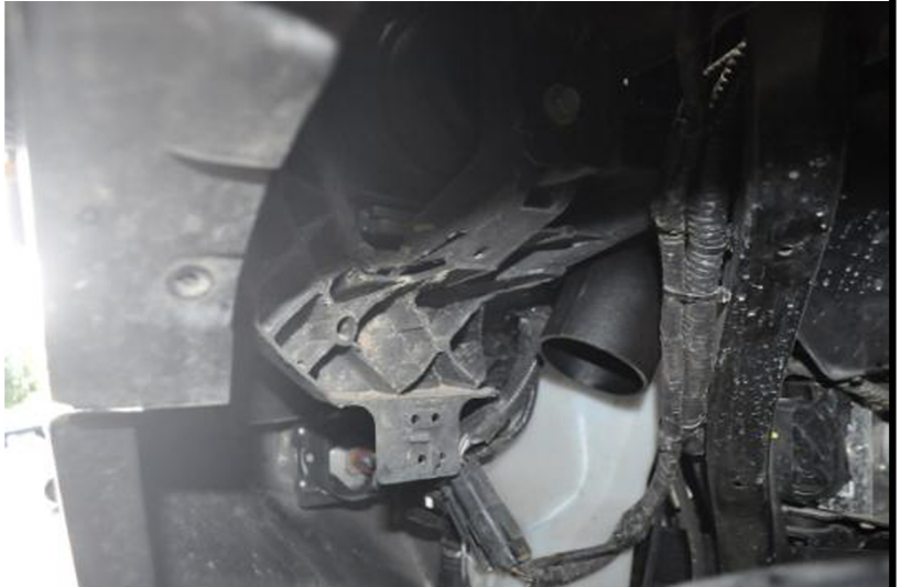
ABOVE: Note the air box adaptor is visible, and there is plenty of room for the hose.
