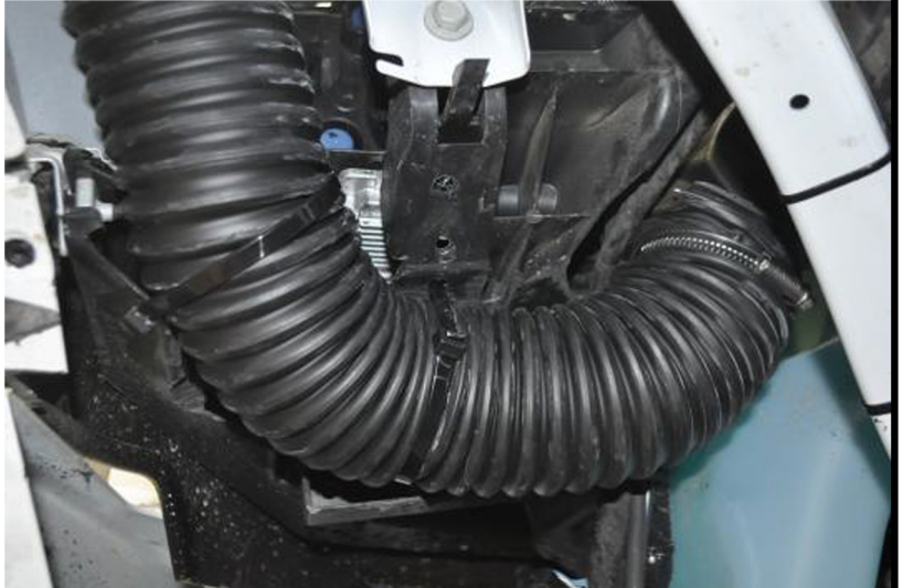
ABOVE: The flexy hose zip tied in the wheel arch BELOW: Don't forget to silicon the air box end of the hose
