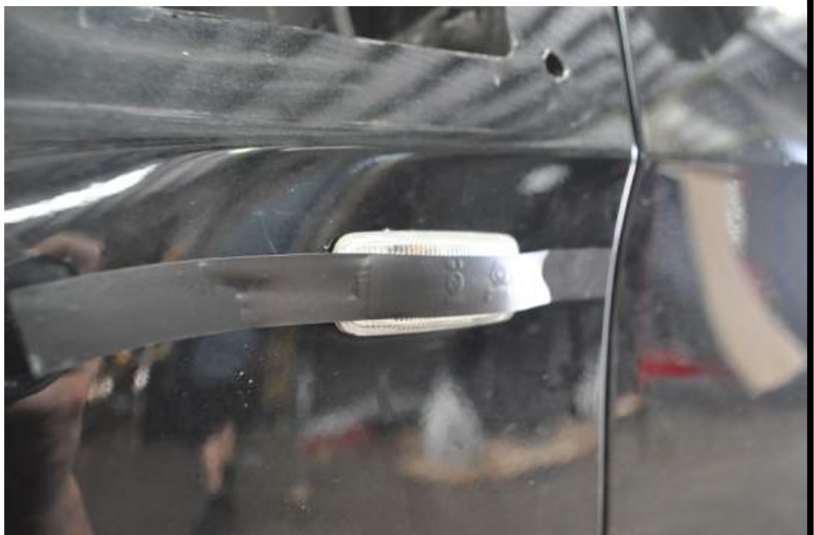
ABOVE: The side indicator removed with tabs trimmed BELOW: Tape holding the side indicator while the silicon sets
