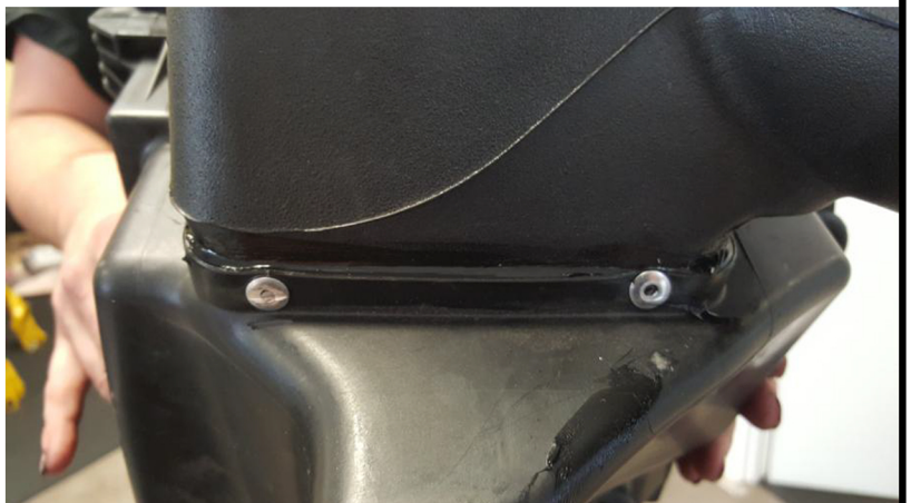
ABOVE: pop rivets joining the air box and connector
