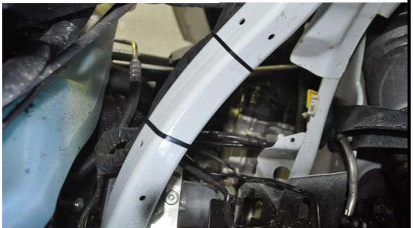
BELOW: The wiring loom to be moved secured to the support
