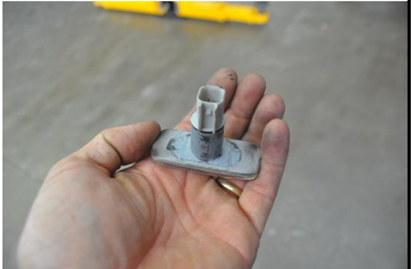
ABOVE: The side indicator removed with tabs trimmed BELOW: Tape holding the side indicator while the silicon sets
