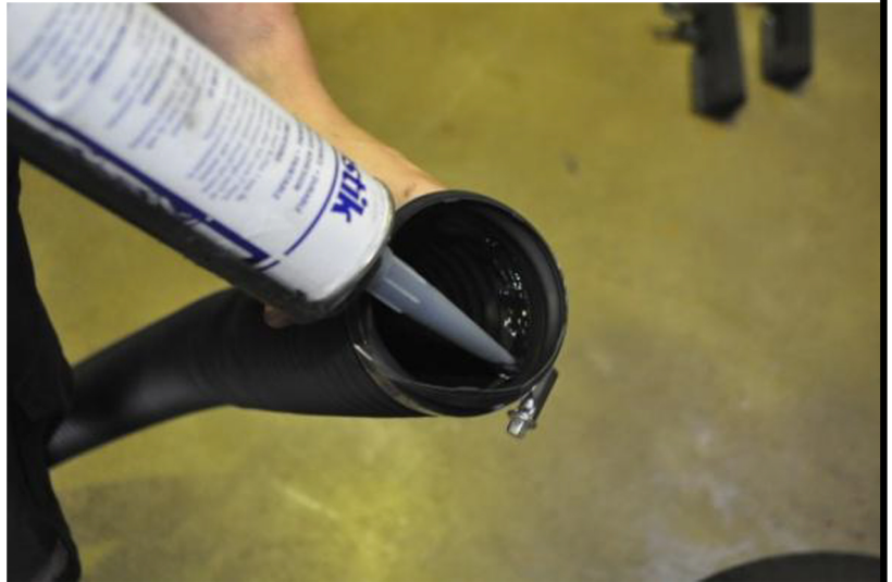
ABOVE: Silicone on the inside of the flexy hose
