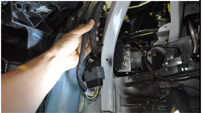
BELOW: The wiring loom to be moved secured to the support
