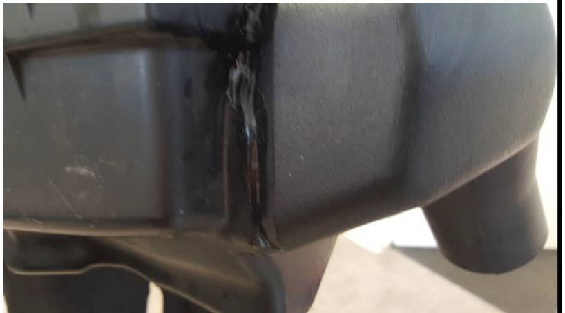
ABOVE: An upper lip on the air box stops the connector from sitting flush BELOW: The connector sitting flush to the air box
