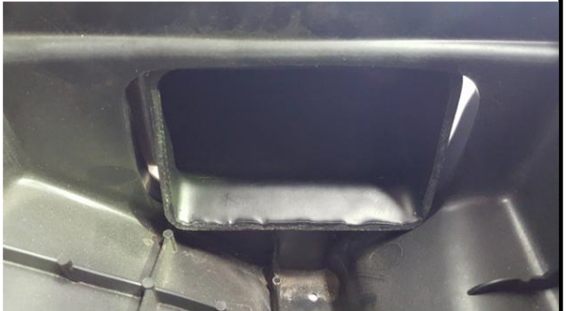
ABOVE: An upper lip on the air box stops the connector from sitting flush BELOW: The connector sitting flush to the air box
