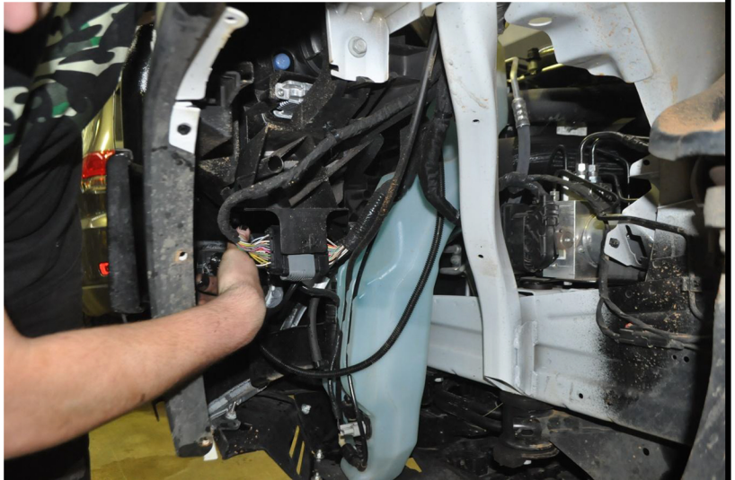
ABOVE: Wheel and innder guard removed BELOW: The wiring loom to be moved
