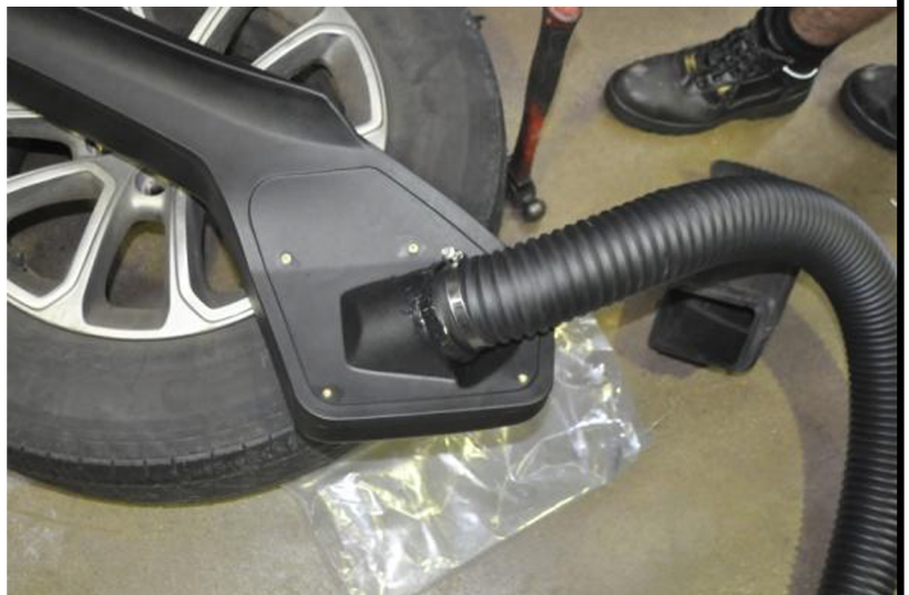
BELOW: The hose attached and clamped to the snorkel body
